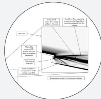
Among other complex applications, Firefly uses Nimbix to simulate how its rockets’ turbine exhaust gas can optimally insulate the critical nozzle extension from the super-heated gas produced by the main engine.
